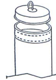
COMPRESSION BAND with disposable top Used in Shaker and Reverse Air Collectors
